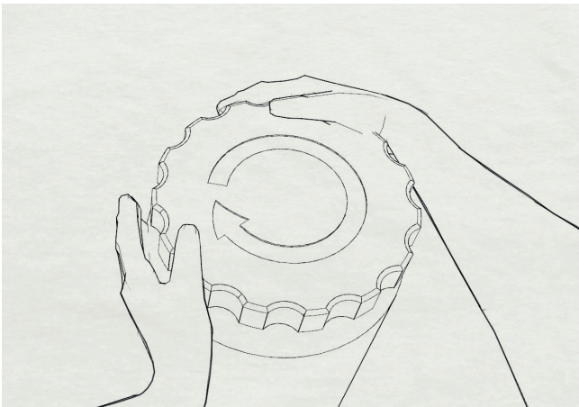
Figure 10 Maximum positions of the wrist should be avoided. The left hand in particular has to be stretched far backwards (dorsal extension).
