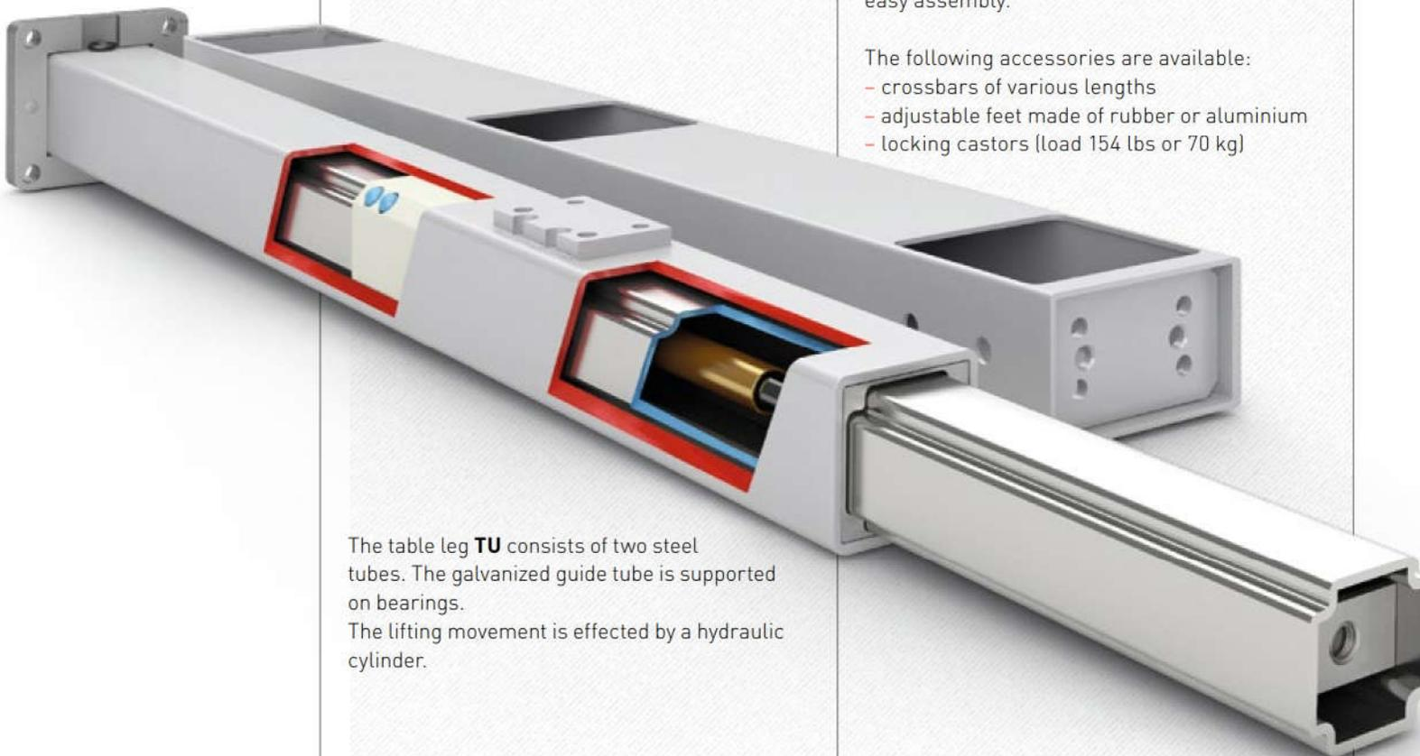
The table leg **TU** consists of two steel tubes. The galvanized guide tube is supported on bearings. The lifting movement is effected by a hydraulic cylinder.
